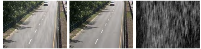
Fig. 1. A frame of a rainy video (left), the rain streaks removal result by the proposed method FastDeRain (middle) and the extracted rain streaks (right). The pixel values of the rain streaks are scaled for better visualization.
