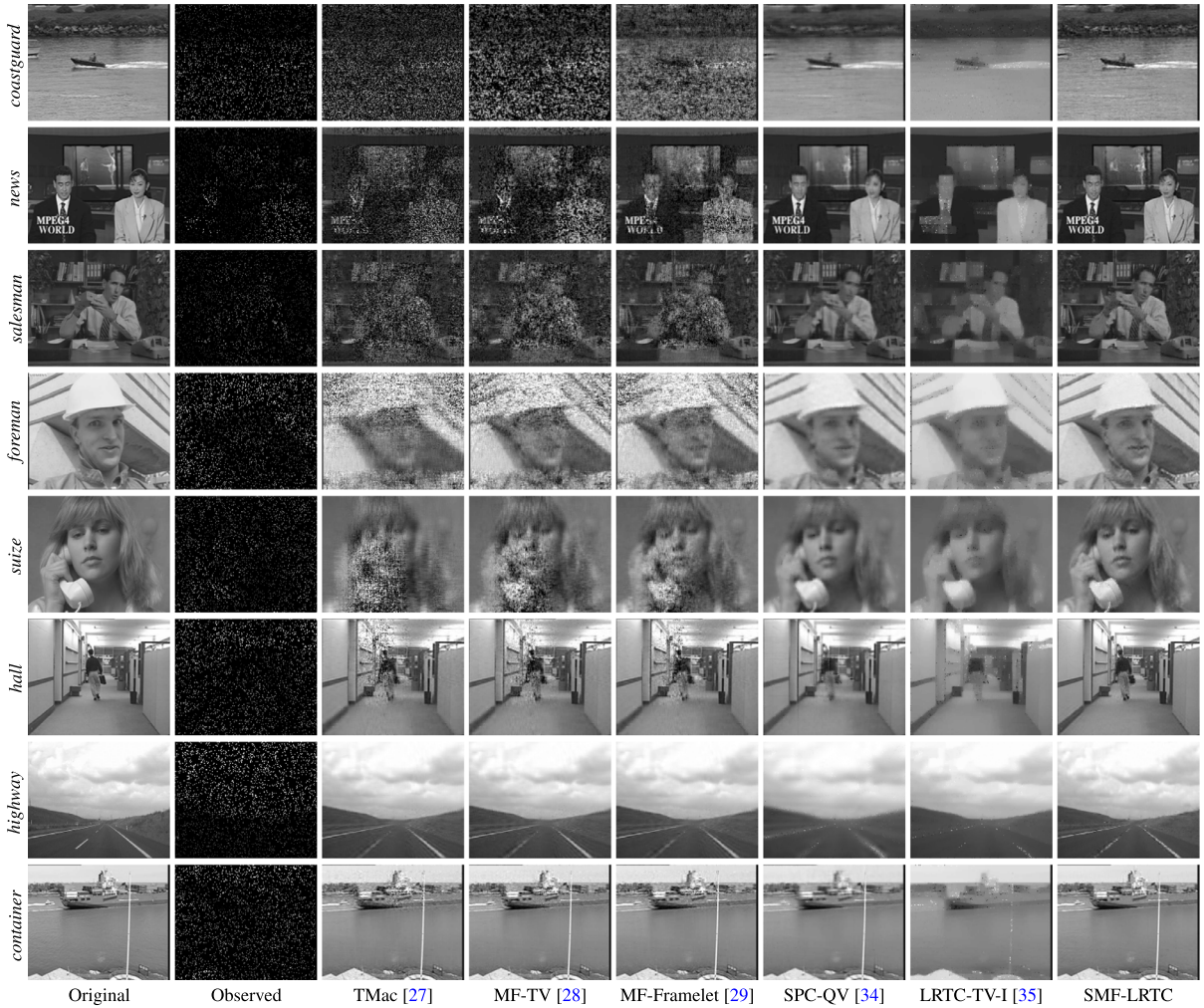
Fig. 3. One frame of the testing videos reconstructed by six utilized LRTC methods with SR = 10\% . From left to right: the original data, the observed data, the reconstructed results by TMac [27], MF-TV [28], MF-Framelet [29], SPC-QV [34], LRTC-TV-I [35], and the proposed method, respectively.
