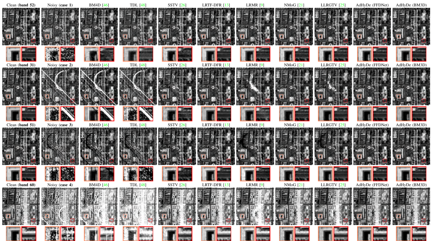
Fig. 5. Denoising result of different bands for Washington dc data with different kinds of noise.
