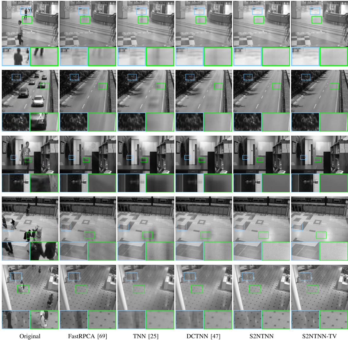
Fig. 6. The separated background by different methods for background subtraction on videos Port ( 144 \times 176 \times 250 ), Highway ( 240 \times 320 \times 200 ), Office ( 240 \times 360 \times 200 ), PET ( 288 \times 360 \times 300 ), and Shop ( 256 \times 320 \times 100 ).
