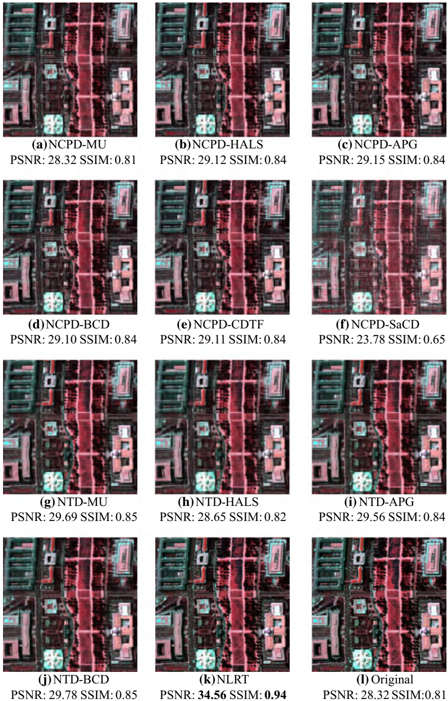
Fig. 7 Pseudocolor images composed of the 113-th, 2-nd, and 16-th bands of the nonnegative low-rank approximations by the different methods when setting the rank 100 on the Washington DC Mall
