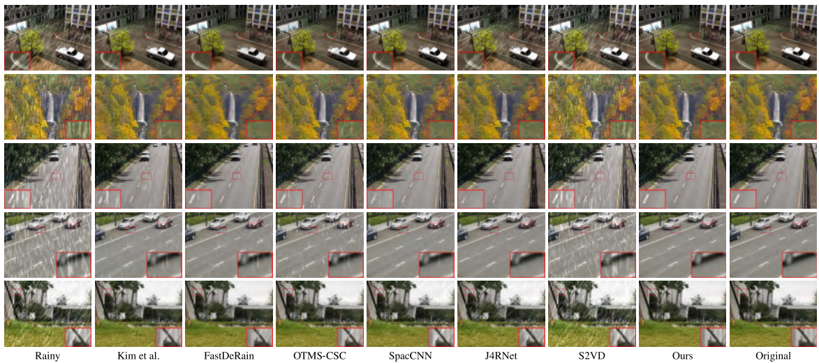
Fig. 6. The deraining results by different methods on simulated data Truck , Waterfall , Highway , Car , and Building in Case 2 . (The images are best viewed in full-screen mode.).
