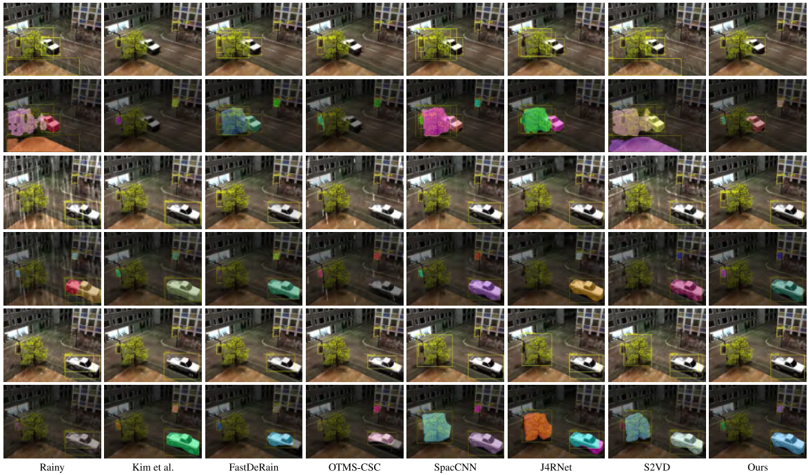
Fig. 14. Three frames of the deraining results (the 1st, 3rd, and 5th rows) by different methods on Truck in Case 1 and the corresponding object detection and instance segmentation results (the 2nd, 4th, and 6th rows) using the mask R-CNN. .
