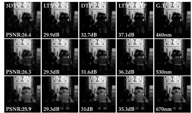
Fig. 2. Three different wave band spectral images ( 128 \times 128 ) were reconstructed by 3DTV, LTNN, DTP, and LTNN–DTP joint priors (5% sampling ratio), respectively.
