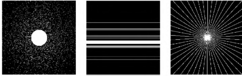
Figure 2. Examples of undersampling masks used in this study. White pixels indicate sampling points. Left: the Gaussian 2D mask. Middle: the Cartesian 1D mask. Right: the radial mask.
